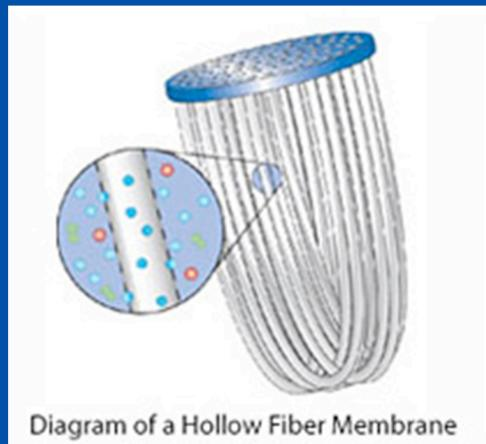
**Diagram of a Hollow Fiber Membrane**
